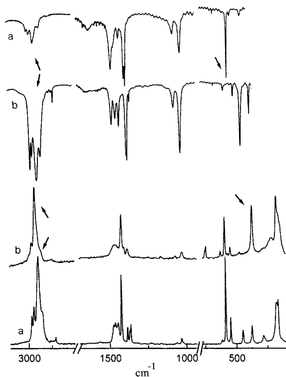
Fig. 1. IR (KBr disk, upper curves) and Raman (crystals, lower curves) of the \text{FeCp}_2^* (a) and [\text{FeCp}_2^*]^+[\text{PF}_6]^- (b) complexes. The arrows show the most significant differences between the spectra of the complexes (see text).
